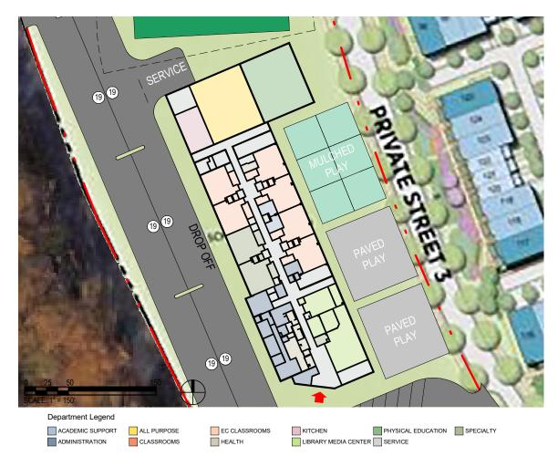
The WMAL site contains a little over 4 acres for development and the main access is provided by Greentree road and newly proposed residential streets. Two curb-cuts have been added for staff parking, service and parent drop off. An additional two curb cuts have been added to provide for bus parking. The 3-level design is efficient in allowing the top two floors to contain required uppergrade classrooms, while early childhood classrooms and specials are placed on the first floor.
